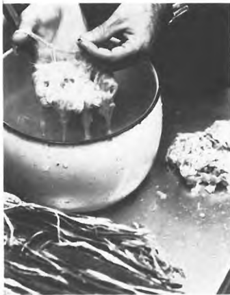
2 After boiling, the strips of inner Gampi bark are picked clean of impurities.
