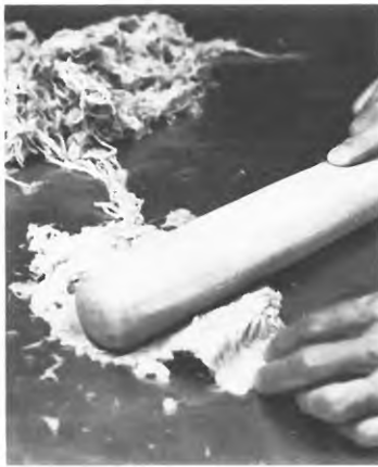
3 The beating of the clean inner Gampi bark is done by pounding the material with a wooden mallet. This process breaks down and macerates the oriental fibers which will be added to the vat with water in preparation for paper-making.
